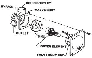
To test operation of Unitherm Governor, place in hot water and watch for movement against spring. If no movement, replace.
